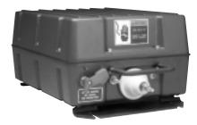
The RF-382A Series couplers efficiently and automatically match the output of 100 to 500 watt transceivers and transmitters to a wide variety of whip, dipole, and long-wire antennas over the frequency range of 1.6 to 30 MHz. Tuning time from memory is less than 200 milliseconds.
